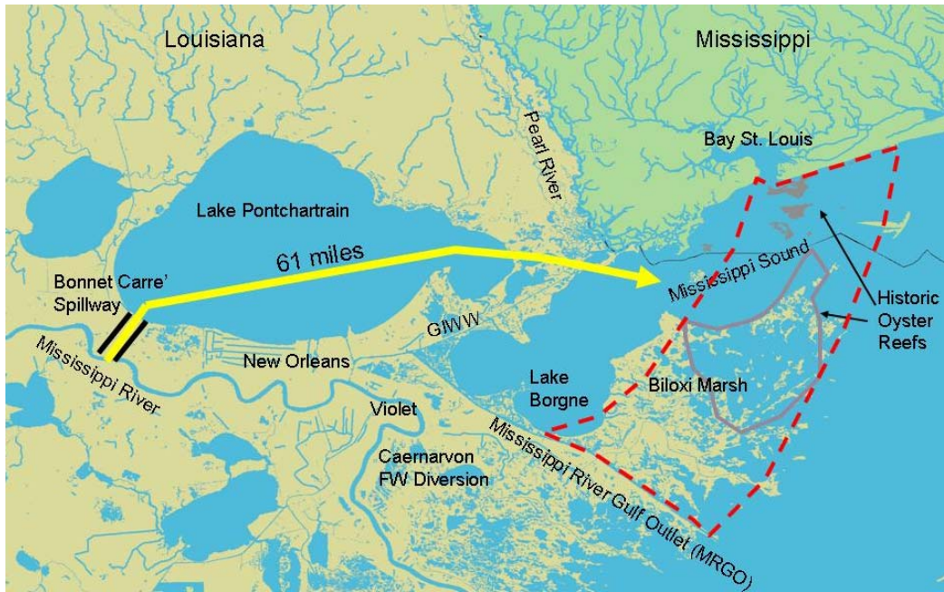
Figure 1: Map depicting the 1984 Feasibility Study’s preferred alternative to construct a new Mississippi River diversion at the Bonnet Carré’ Spillway. The project assumed the MRGO would remain open and continue to elevate salinity in Lake Borgne. The target benefit area for oyster enhancement is outlined in red. (source, 1984 Feasibility Study 2 ). Historic reefs are shown in gray.
