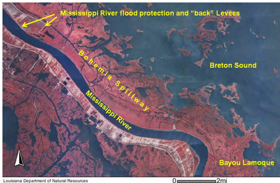
Figure 1: Bohemia Spillway area is east of the Mississippi River downstream of the terminus of the Mississippi River levee (source basemap: SONRIS CIR 2005).
